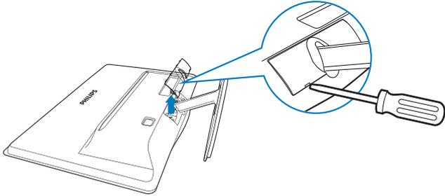
2. Remove 4 screws and then remove the base from the monitor.
