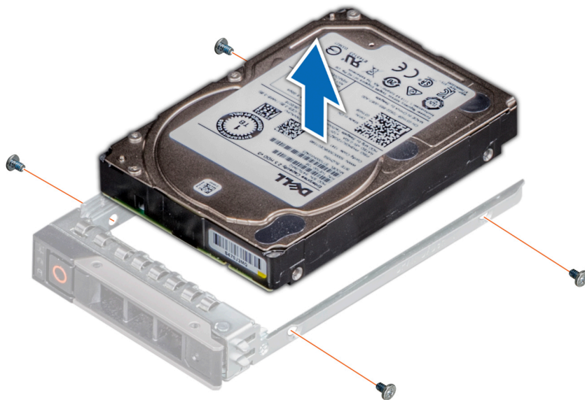
Figure 52. Removing the drive from the drive carrier
