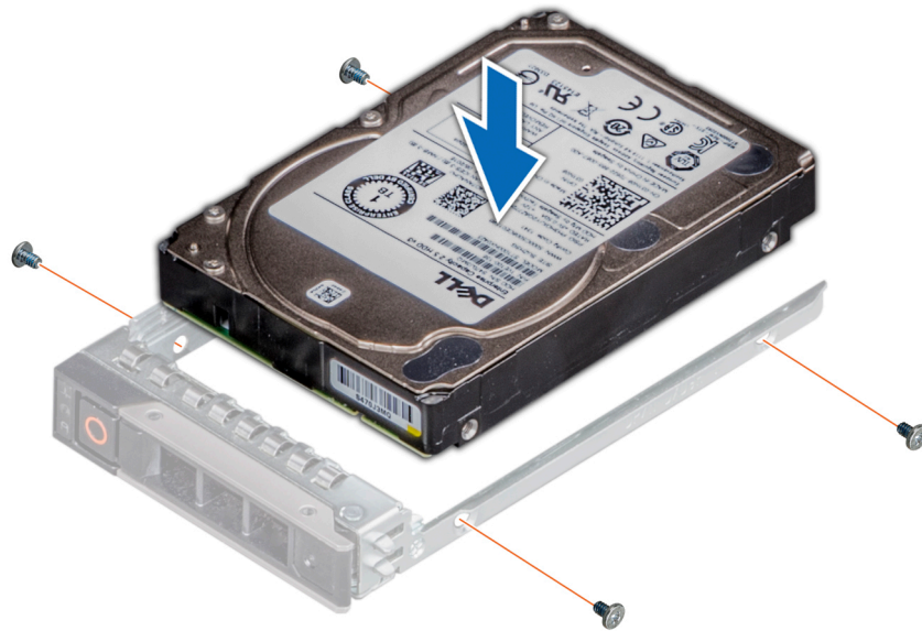
Figure 53. Installing a drive into the drive carrier
