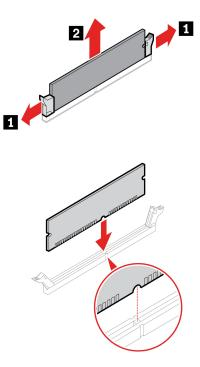
**Note:** During the installation, ensure that you align the memory module to the slot and press down on both ends until the latches are fully engaged with a click.
