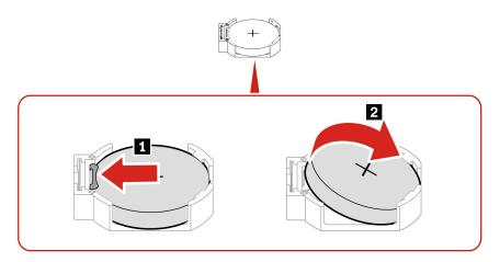
**Note:** After installing a new coin-cell battery, reset the system date and time in the UEFI BIOS menu.
