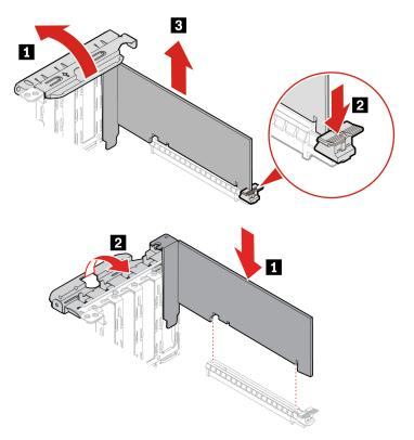
**Note:** During the installation, ensure that you align the PCI-Express card to the slot and press down until the latch is fully engaged with a click.
