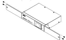
2. Align the mounting brackets' screw holes with that of the front of the rack, and secure the unit onto the rack using 2 self-supplied screws.
