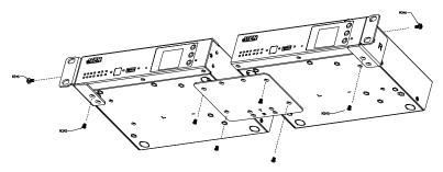
3. Align the mounting brackets' screw holes with that of the front of the rack, and secure the units onto the rack using 4 self-supplied screw.
