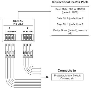
Connect to devices for controlling and receiving status messages from them. For bi-directional RS-232 control, the transmit (TX), receive (RX) and ground (GND) terminals must be wired on both the VK1200 / VK2200 and the device connecting.
