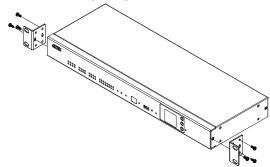
2. Align the mounting brackets' screw holes with that of the front of the rack, and secure the unit onto the rack using 4 self-supplied screws.
