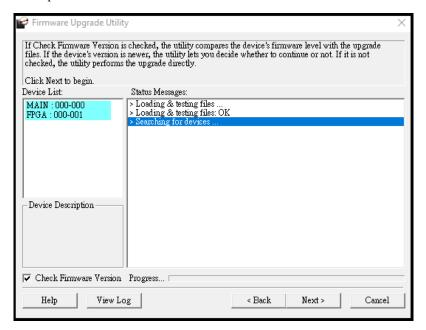
4. Click **Next** to perform the upgrade. The Status LEDs SDI, HDMI, and power will flash while the upgrade is in process.
