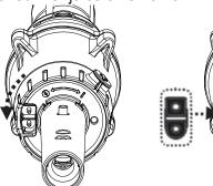
2. Connect the USB charging cable to the USB charger, then plug the USB charger into the power source. Once the electric vacuum begins to charge, the indicator light will turn red. Normally, it takes about **4.5 - 6** hours to reach a full charge. The indicator light will turn green once the electric vacuum is almost fully charged.
