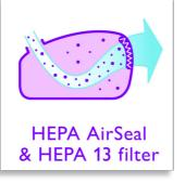
This Philips vacuum cleaner has been designed in such a way that all the air taken in is passed through the washable HEPA 13 filter (99.95% filtration) before it is exhausted. No escape is possible.
