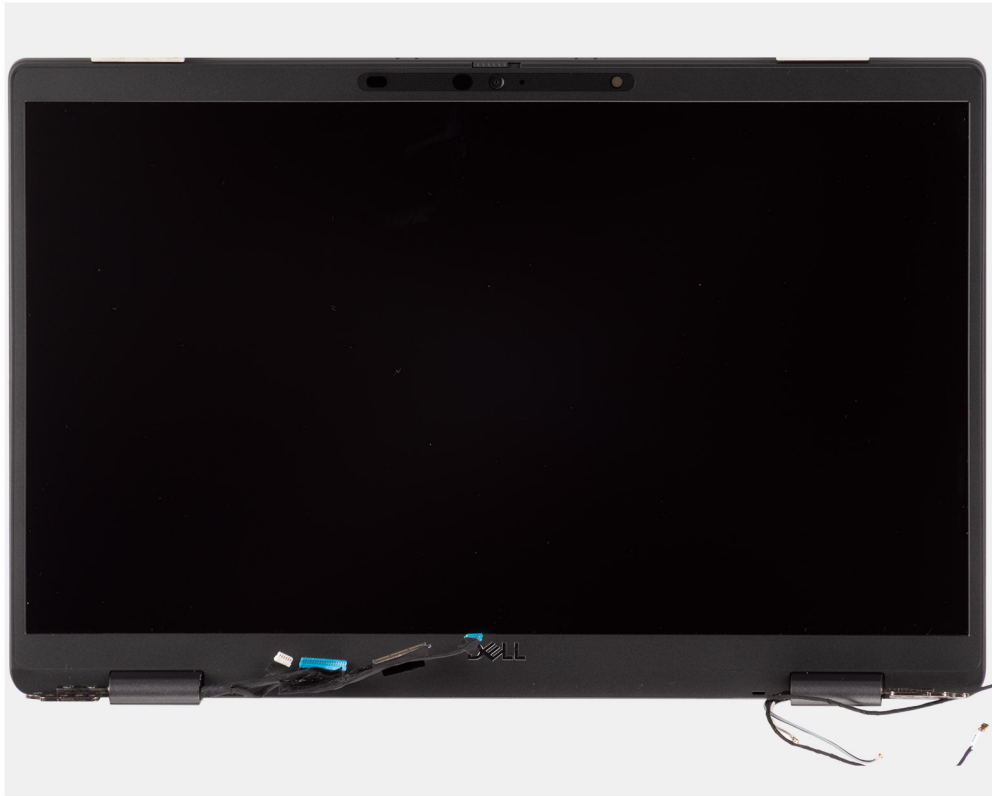
Figure 1. Display assembly with antennae cables
