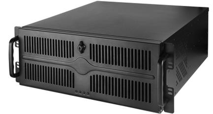
The **UNC-409S-B** is a compact 4U ATX rackmount case, with a short depth of only 482mm, while able to install **ATX motherboards**. The robust build quality with 1.2mm thick SECC steel ensures good protection of the hardware and serves as a reliable and flexible long-term solution. Sufficient cooling options with 2x 120mm front and 2x 80mm rear installation of optionally available fans are provided. Two fast **USB 3.1 ports** in the front panel add to the features on offer with this chassis.
