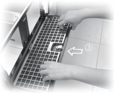
1. Pull out the Filter bracket and remove the used filter.
