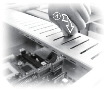
4. Affix the hold down clamp with thumb screws
