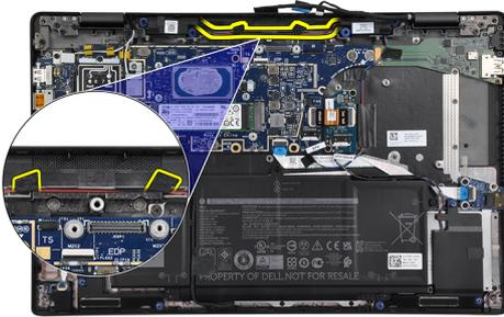
5. Replace the display cable bracket on the eDP connector on the system board.
