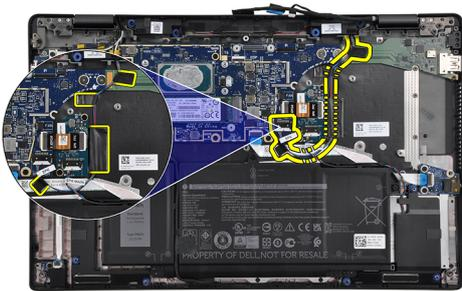
4. Replace the tweeters and palmrest antenna assembly into its slot in the palmrest assembly.
