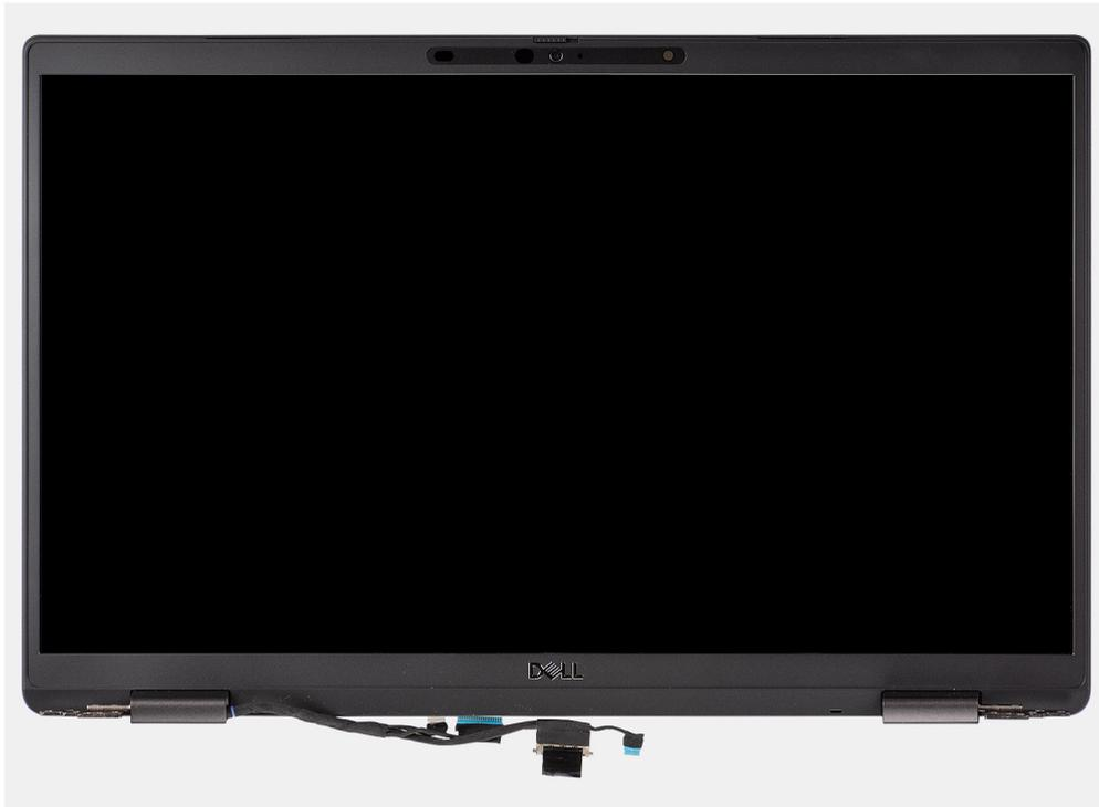
**Figure 1. Display assembly without antennae cables**
