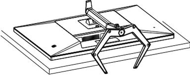
2. While keeping the release button pressed, tilt the base and slide it out.
