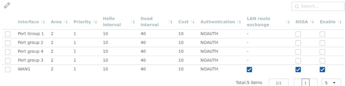
The image shows a screenshot of a web interface for OSPFv2 configuration. It features a table with columns for Interface, Area, Priority, Hello interval, Dead interval, Cost, Authentication, LAN route exchange, NSSA, and Enable. There are checkboxes for each row and a search bar at the top right. Below the table, there are pagination controls showing 'Total: 5 items', '1/1', and a dropdown menu set to '5'.
