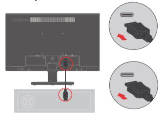
5. Plug the power cord into the display, and then plug the display power cord and computer cord into a grounded power outlet.
