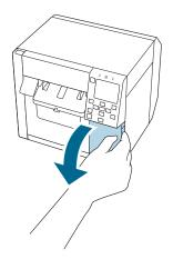
Press the lever down to remove the used ink cartridge.
