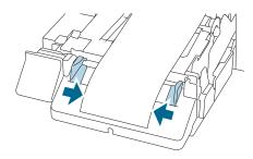
16 Raise the lock lever of the paper ejection guides until it clicks into place.
