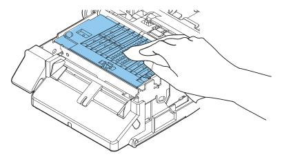
Use cotton swabs to clean the holes and around the holes. If the holes are blocked, be sure to remove the dirt to unblock the holes.
