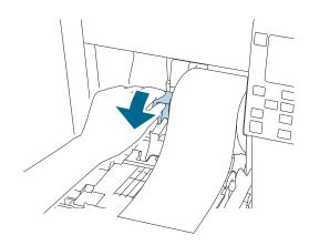
According to the paper width, open and/or close the platen shutters.
