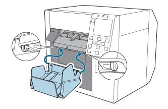
Pull the lever at the bottom right of the OT-PT40 to release the lock.
