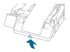
Pull out the leading edge of the roll paper, and then close the front cover.
