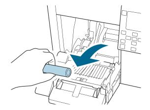
Attach the OT-WA34 by inserting it into the grooves inside the front cover.
