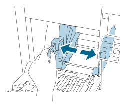
6 Lower the lock lever of the roll paper guides.
