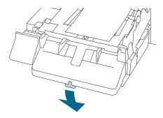
Slide the paper ejection guides outward.
