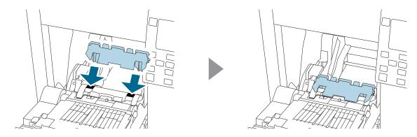
According to the paper width, open and/or close the platen shutters.
