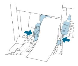
Lower the lock lever of the roll paper guides.
