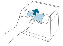
Remove the paper feed guide, and then close the rear cover.
