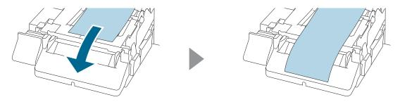
Hold down the paper by hand, and slide the roll paper guides against the paper.
