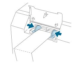
Lower the lock lever of the fanfold paper guides.
