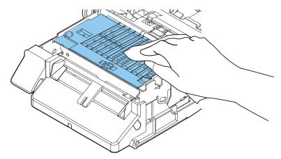
Use cotton swabs to clean the holes and around the holes. If the holes are blocked, be sure remove the dirt to unblock the holes.
