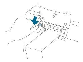
Insert the leading edge of the paper with the printable side face up.
