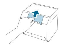
Raise the lock lever of the fanfold paper guides.
