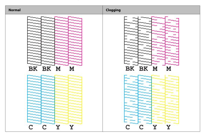
When the printed patterns show the nozzle clogging state, run a head cleaning.
