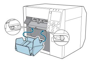
Pull the lever at the bottom right of the OT-PT40 to release the lock.
