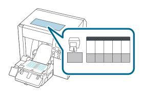
Lower the lock lever of the paper ejection guides.
