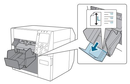
Push in lever at the bottom right of the OT-PT40 to lock it in place.
