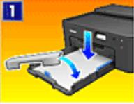
1. Load paper into the cassette, and then insert the cassette into the printer.
