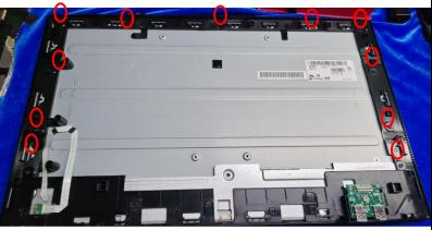
Remove the screws on the middle frame
