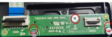
Remove the 3pcs screws on the keyboard
