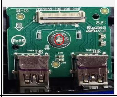
Remove the screw on the usb board
