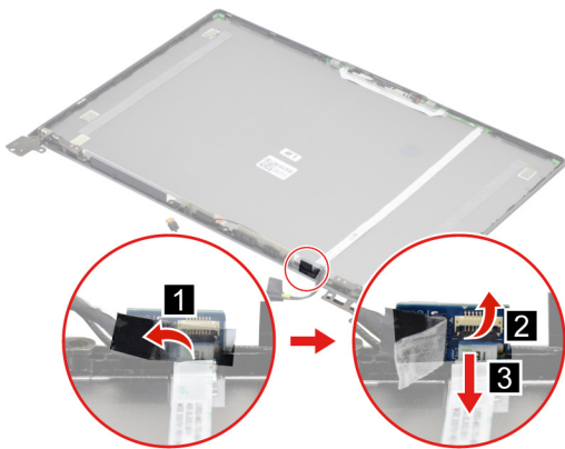
Figure 46. Peel off the tape and then disconnect the camera cable from the trans board
