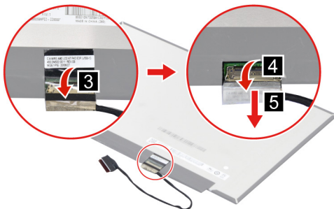
Figure 42. Peel off the tape and then disconnect the EDP cable from the LCD panel
