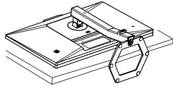
2. While keeping the release button pressed, tilt the base and slide it out.
