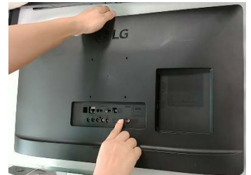
Turn it upside down and remove the back cover by pressing antenna jack.
