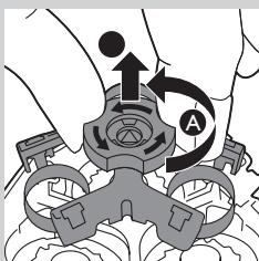
**4 Turn the lock anticlockwise (A) and remove the retaining frame (B).**
