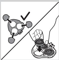
Note: Make sure that the projections of the shaving heads fit exactly into the recesses.
