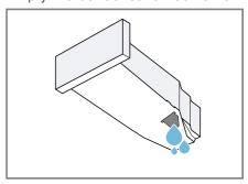
Check the condensation container filter  $\rightarrow$  *Page 44* regularly and clean the filter if it is dirty. Make sure that you insert the condensation container before operating the appliance.
