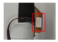
S10 Disassemble USB FFC from USB BD and I/F BD
