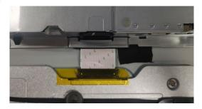
S14 Disassemble LVDS cable from Panel
