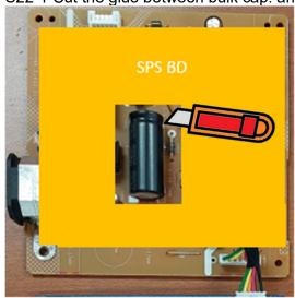
S22-2 Ensure cutting path within the glue, don't touch bulk cap. or PCB
