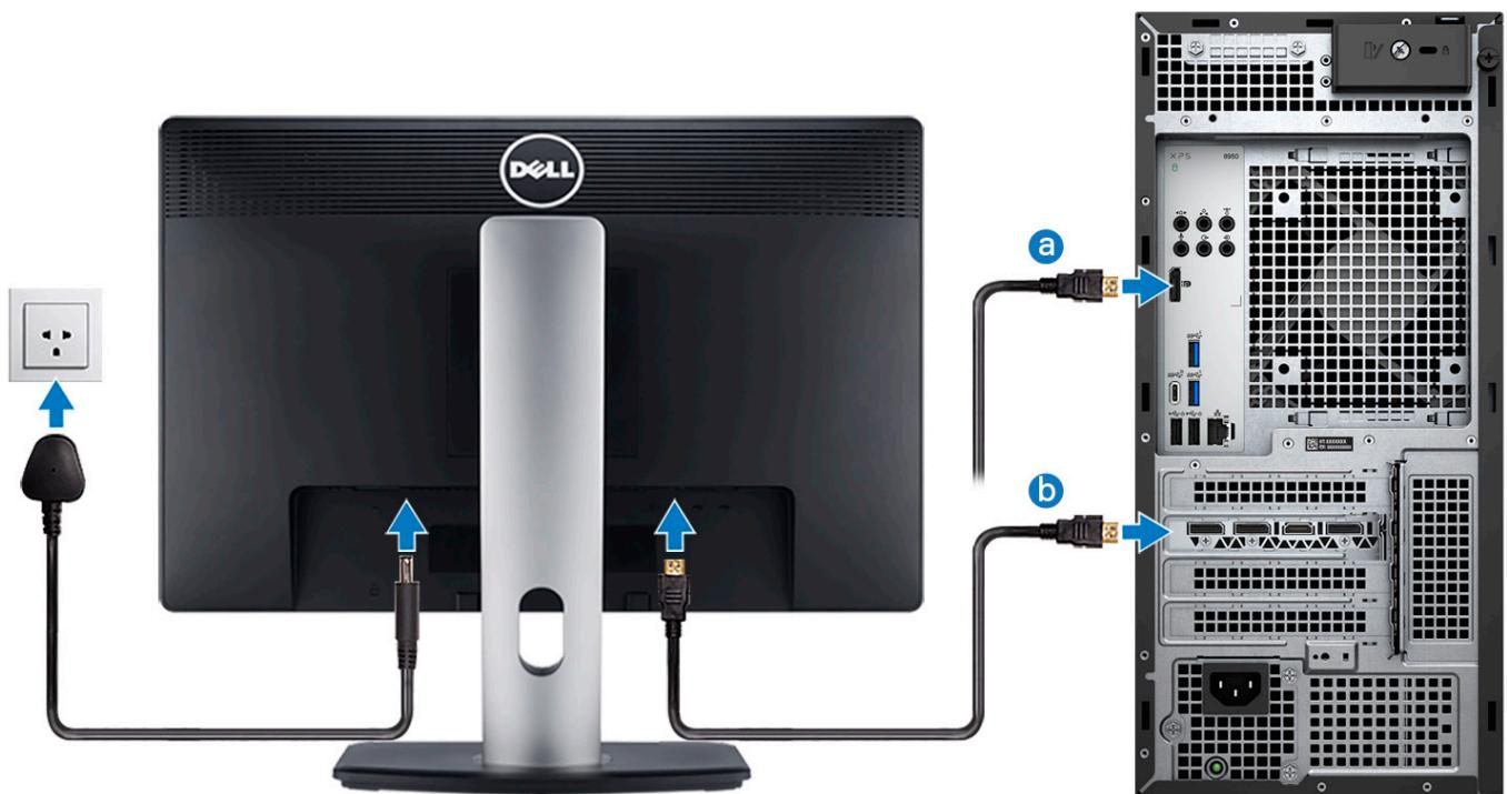
**i** **NOTE:** There are different connection points for your display depending on whether your computer has a discrete graphics card installed.
