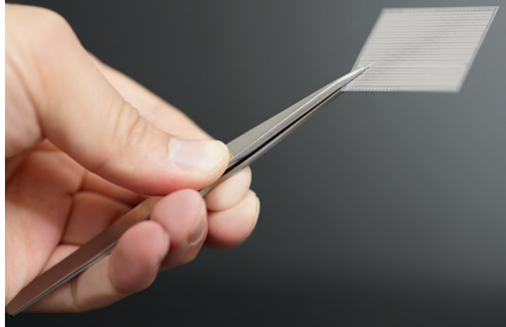
40µm Piezoelectric element
