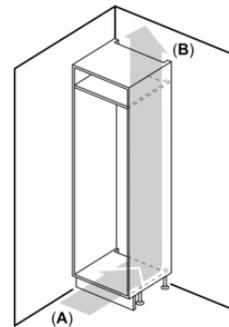
A: Air inlet  $\geq 200$  cm<sup>2</sup>; Ventilation options
