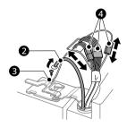
3 Rotate the hinge lever S counterclockwise. Lift the top hinge G free of the hinge lever latch **7**.
