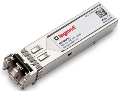
Linksys MGBSX1 Compatible 1000Base-SX SFP Transceiver (MMF, 850nm, 550m, LC Duplex, DDM, I-Temp)
