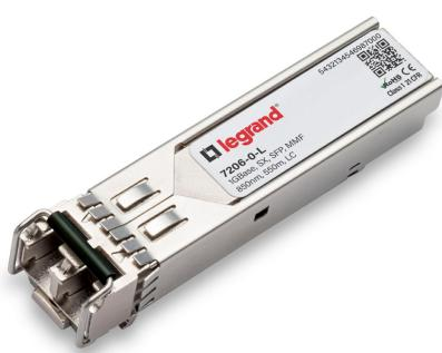
Omnitron 7206-0 Compatible 1000Base-SX SFP Transceiver (MMF, 850nm, 550m, LC Duplex, DDM, I-Temp)
