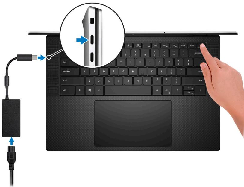
**i** **NOTE:** You can charge your system by connecting the power adapter to one of the two Thunderbolt 4 (USB Type-C) ports that are located on the left side of your computer or to the USB 3.2 Gen 2 (Type-C) port located on the right side of your computer.
