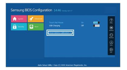
4 The Battery Calibration function is activated and the battery is forcefully discharged. To stop the operation, press the **Esc** key. This operation requires 3–5 hours depending on the battery capacity and the remaining battery charge.
