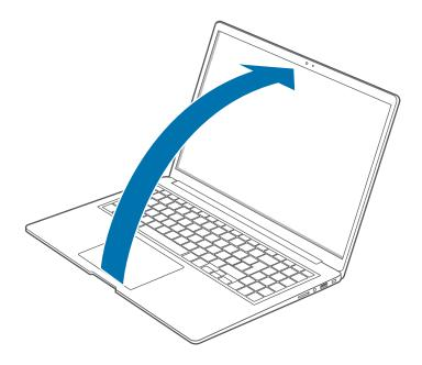
3 The computer turns on automatically when the display panel is opened.
