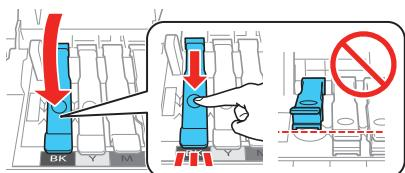
**Note:** Replace the bottle cap and tighten it.
