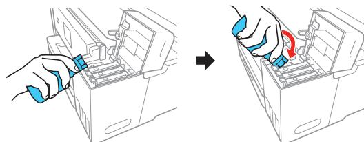
**Note:** Refer to the color-coded sticker on the ink tank unit to identify the color of each tank. Do not force the bottles into position; they are keyed for each color.
