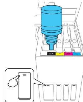
**Note:** If ink does not flow from the bottle, lift and reinsert the bottle.
