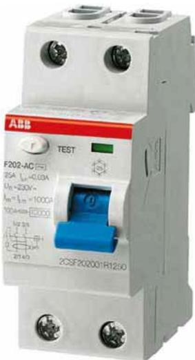
A residual current device (RCD,) is the generic term for a device that monitors the current in the line conductor and the neutral conductor of a circuit in an earthed system.
