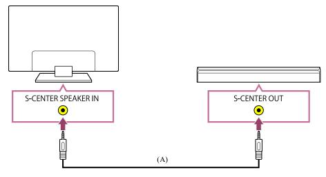
(A) TV centre speaker mode cable (supplied with sound bars that have S-CENTER OUT terminals)
