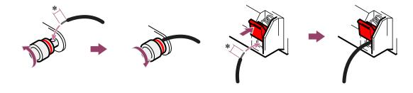
\*Strip about 10 mm (13/32 inches) of insulation from the speaker cable at each end.
