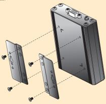
2. Screw the mounting brackets to the wall.
