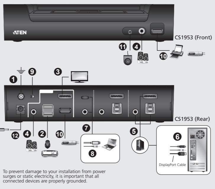
To prevent damage to your installation from power surges or static electricity, it is important that all connected devices are properly grounded.
