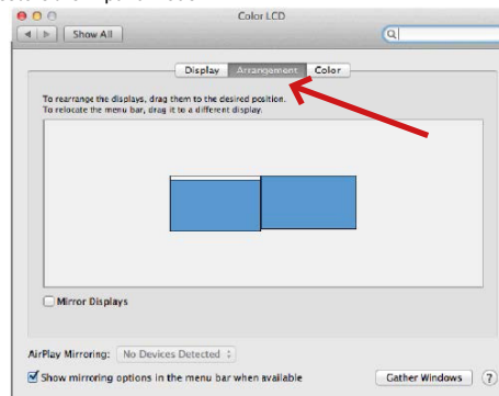
Expand mode: The arrow indicates the possibility of positioning the connected monitor relative to the Mac monitor.
