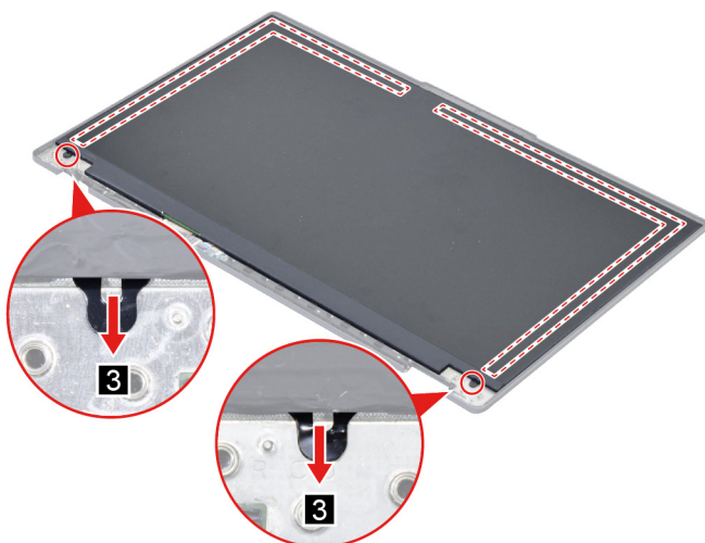
Figure 35. Remove the two pieces of removable tape
