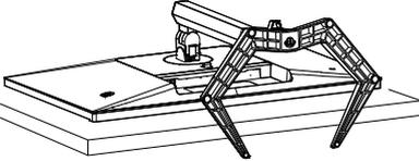
2. While keeping the release button pressed, tilt the base and slide it out.
