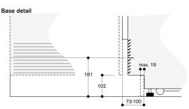
Based on the standard appliance height, the height of the plinth is 102 mm. Maximum plinth thickness 19 mm.
