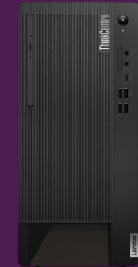
Connect up to 4 independent displays and industry-specific equipment with onboard ports, which include 5x USB ports, 1x HDMI, and 2x DisplayPort ports. Plus, it has an array of optional ports including 1x Thunderbolt™ 4 and 4x USB-C ports for transferring data at lightning speed.
