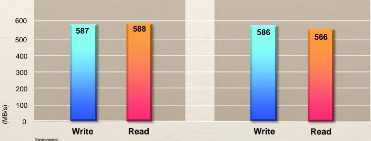
NAS | TS-410E, QTS 5.0, 4 x Samsung 860 Pro 512GB, RAID 5, thick volume PC | Windows Server 2019 Standard, Intel Core i7-6700 3.4 GHz, 32GB RAM
